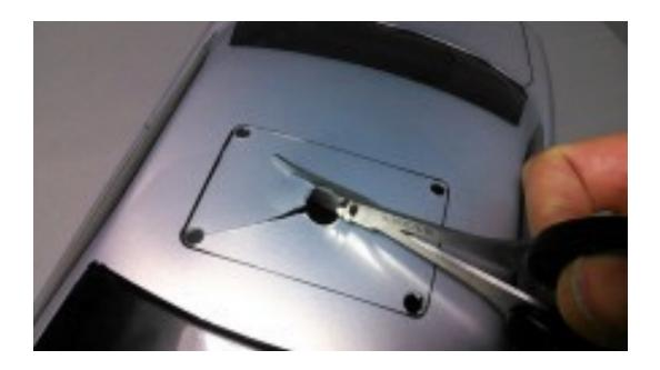
And bend slowly the 4 pieces downwards and upwards so that the material will break loose.
