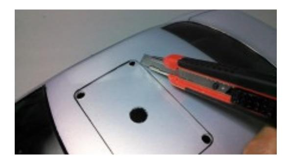
Cut with a scissor from the inside to the 4 holes at the corners.
