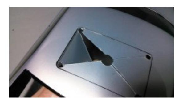
Check if the frames will fits nicely, if not, grind or use fine sandpaper to make it fit. Use it anyway to make your cut smooth at the end.
